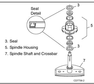
Figure 16. Spindle Disassembly
